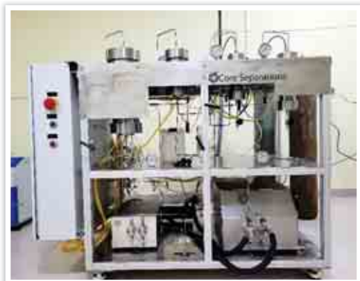
Supercritical Fluid Extractor
